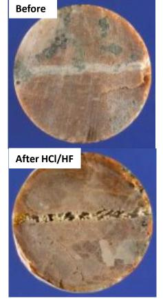
Fracture filling Clays, Quartz & Carbonates
