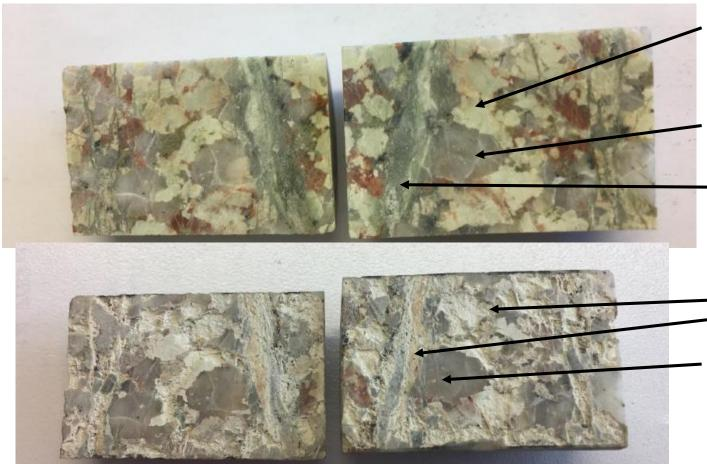
Secondary illite (clay bearing K) located in the Damage Zone (**DZ**) around the Quartz Vein (**QV**) Sample @1674m
