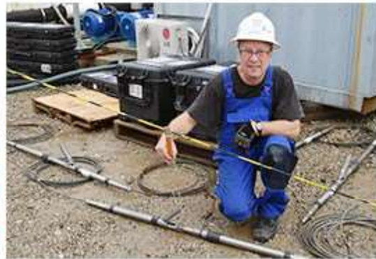
Testing of the geophone chain at the surface.
