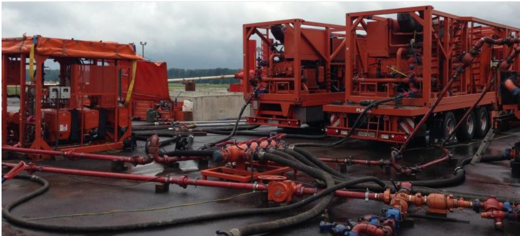
Fig. 20 Surface circuits for the preparation and the mixing of acids for chemical treatment at Rittershoffen geothermal site (France). ©és
