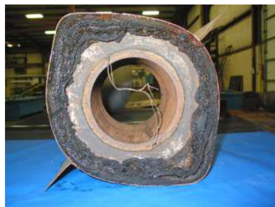
Figure 13: Expansion of a Swell packer in a lemon shape hole, courtesy of TAM international, Inc.
