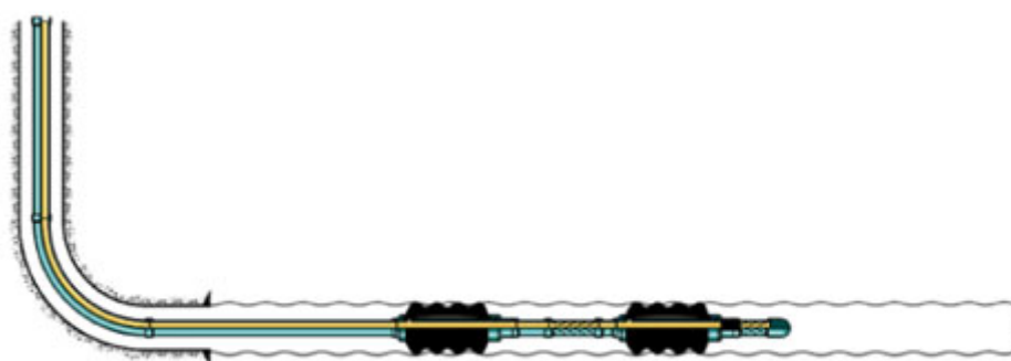
The PosiFrac Straddle System is designed for multiple fracturing treatments in one run.
