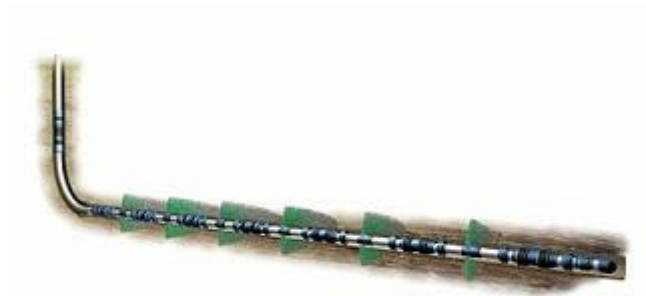
Figure 5: Example of a multi-frac system, courtesy of Packer Plus Energy Services Inc.
