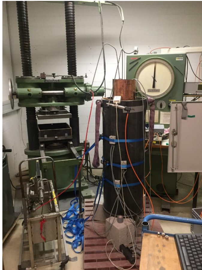
Figure 23: The on-going swelling benchmark test in a cylindrical shape.
