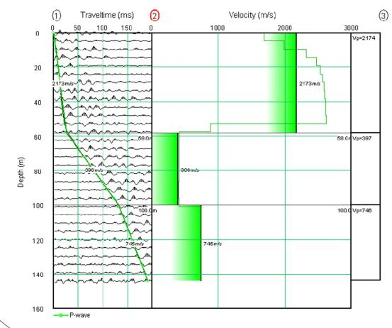
Shallow drilling was also used to determine velocity laws in the shallow layers of the subsoil. This data can be particularly useful for the construction
