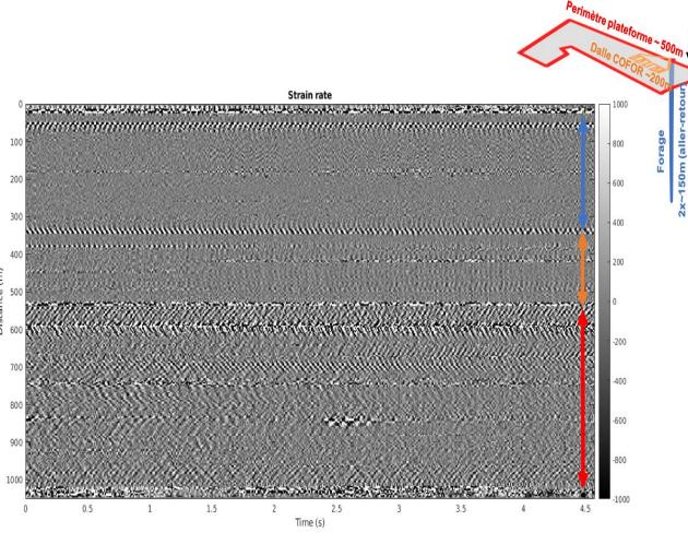
As part of a deep geothermal project, usually made up of at least 2 wells, the drilling machine remains on the platform for several months. The advantage of the optical fiber placed into the concrete is to monitor the state of stress of the concrete slab and anticipate possible concrete failure that can be dramatic for a project.
