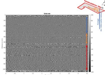
As part of a deep geothermal project, usually made up of at least 2 wells, the drilling machine remains on the platform for several months. The advantage of the optical fiber placed into the concrete is to monitor the state of stress of the concrete slab and anticipate possible concrete failure that can be dramatic for a project.
