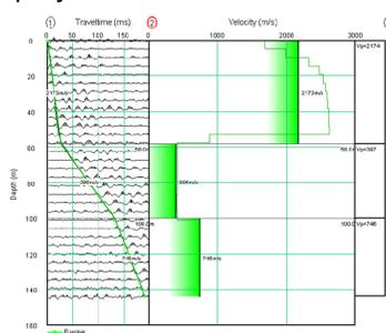
Shallow drilling was also used to determine velocity laws in the shallow layers of the subsoil. This data can be particularly useful for the construction of a velocity model in order to correct static errors in the context of the relocation of microseismic events. It can also be used as an antenna to detect possible microseismic events.
